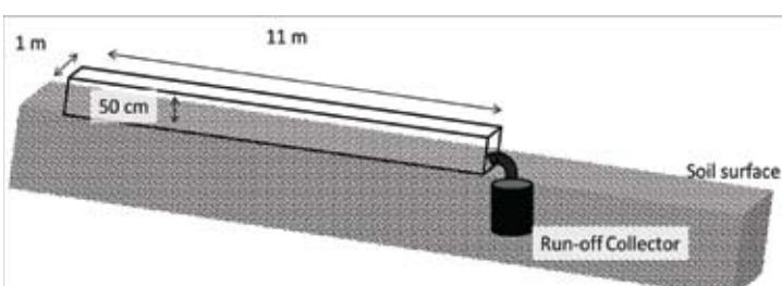
Fig. 2. Dimensions and setup of equipment used for measuring run-off in the study area.
